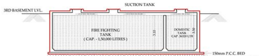
SECTION THROUGH UNDERGROUND WATER TANK
